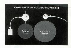
Regardless, the alignment of the applicator roller and metering roller is important, as is the total indicated runout (TIR) of the rollers.
